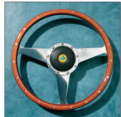
Mark Three with plain spokes, dished version. Shown with black ABS plastic horn control and badge.
